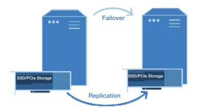
SIOS SANIess cluster synchronizes high performance local storage for high availability without the cost, complexity or single point of failure risk of shared storage.
